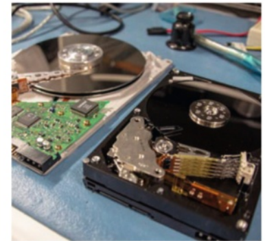
▲ Hard disk internals are sometimes so fragile that a speck of dust could permanently destroy data
