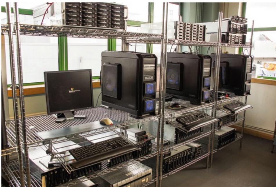
▲ A dedicated suite of enterprise-class systems is used to reconstitute damaged RAID arrays
